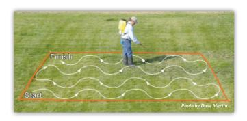
**STEP 3.** Time the number of seconds it takes to spray the measured area uniformly with water using gentle side-to-side sweeping motion with the spray wand similar to spray painting a home or automobile. Record the number of seconds required to spray the area. During application be sure to maintain a constant sprayer pressure and cover the entire area uniformly one time. **You should repeat step 3 at least twice and use the average of the two times.**
